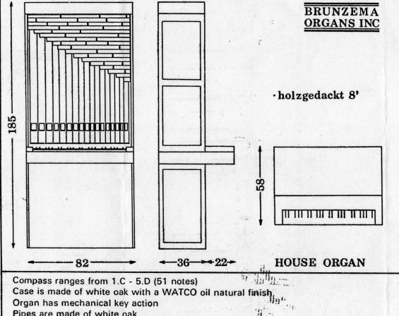
Pipes are made of white oak Keyboard is made of rosewood with ebony sharps
