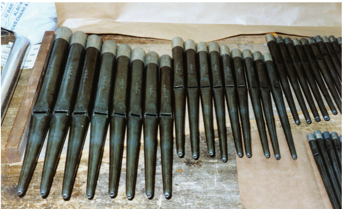
GREAT MIXTURE: rank II Hill 1871 marks on upper lip in ink HNB 1963 marks scribed halfway up front
